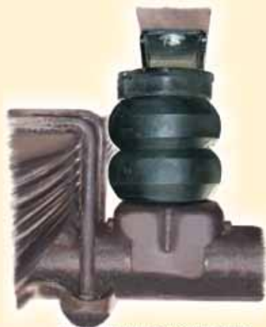
Typical Timbren SES kit installed
