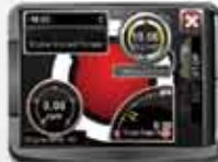
Four tools in one! "Performance Programmer", "Virtual Gauge Monitor", "Virtual Drag Tree" and "Diagnostic Code reader".
