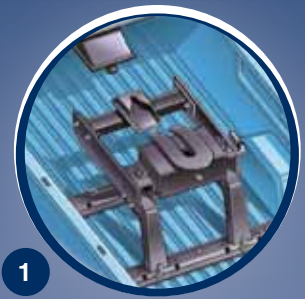
Fifth wheel hitch with BedSaver™ in place.
