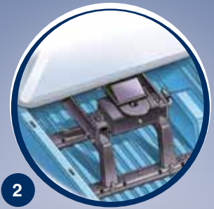
Fifth wheel kingpin fails to seat properly and slips off the hitch.
